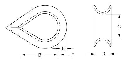
FIGURE 2. Type II, split oval, light fiber and wire-rope thimbles.
